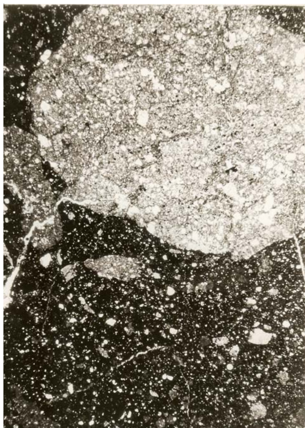
Figure 6: Photomicrograph of thin section 14307,41 with large clast of impact melt breccia. S71-38802. Field of view is ~1.5 cm.
