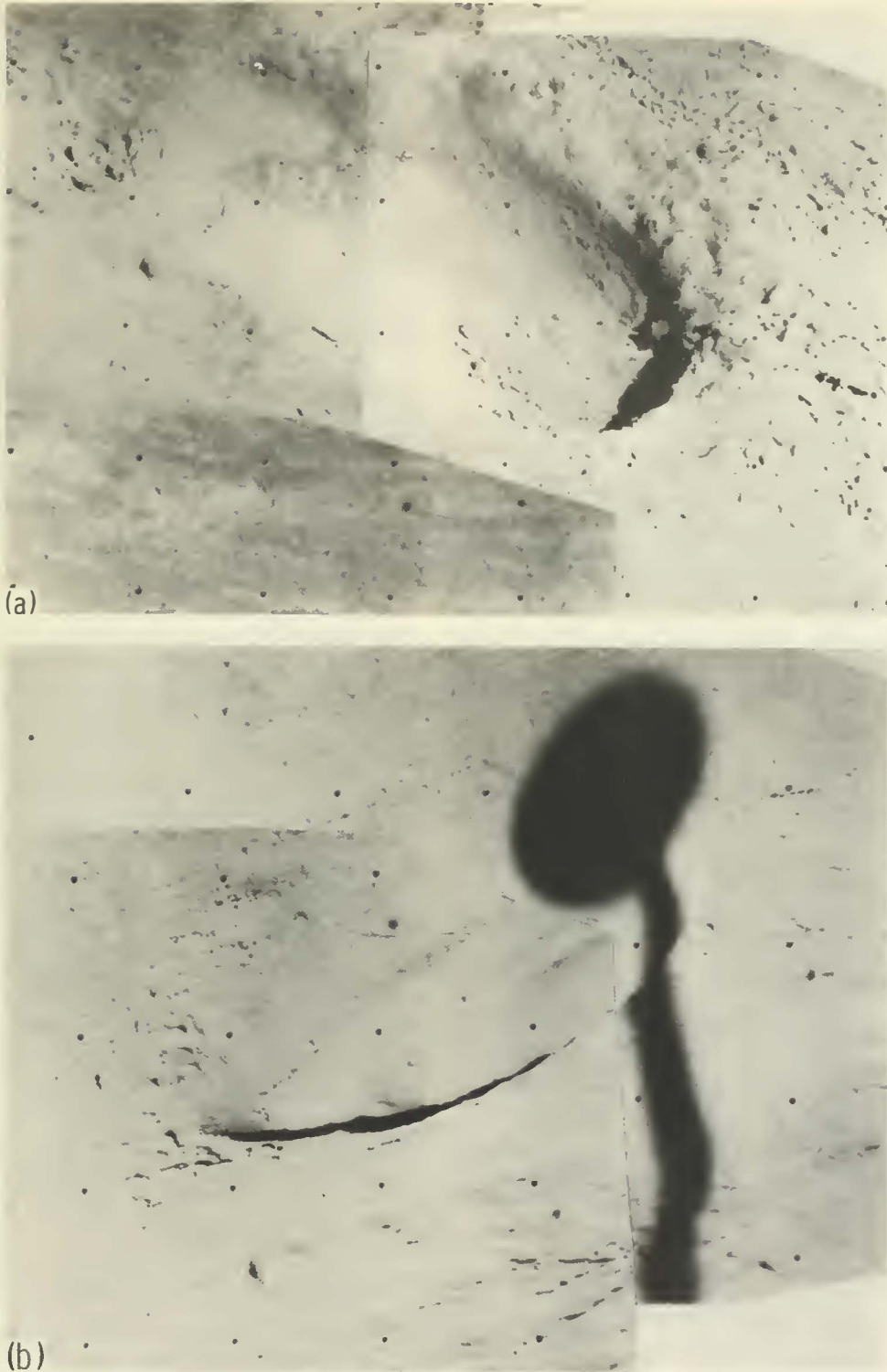
FIGURE 4-9.—Surveyor VI footpad imprints made during initial landing, as seen from posthop position. (a) Footpad 2 imprint (Nov. 17, 1967, Catalog 6-SE-39). (b) Footpad 3 imprint (Nov. 22, 1967, Catalog 6-SE-38).
