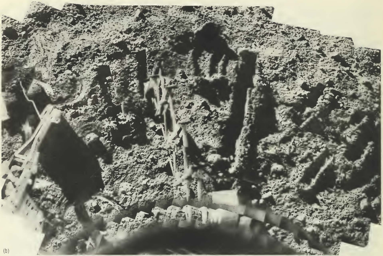
(b) Narrow-angle mosaic of Surveyor VII pictures showing sensor head in place on a lunar rock (sample 2). The surface sampler is seen in the process of digging the second of three trenches at the site of alpha-scattering sample 3. The sample 1 location at the lower
