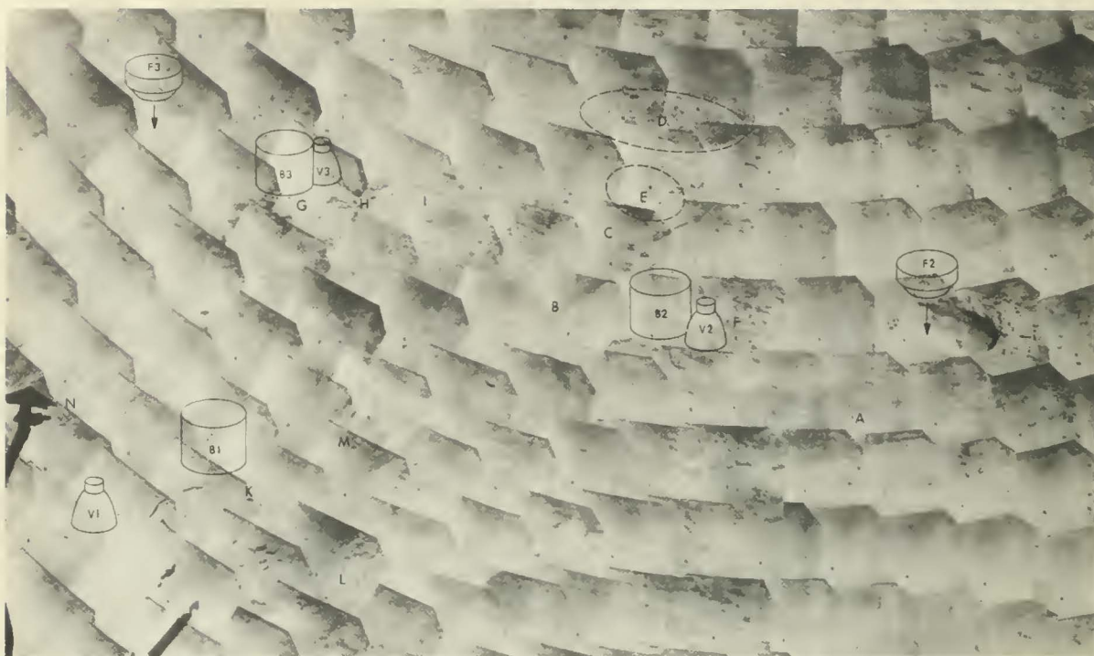
FIGURE 4-22.—Mosaic of posthop, computer-processed pictures showing the (1) approximate locations of the crushable blocks and vernier engines before liftoff for the hop; (2) the images of footpads above their final imprints made during the original landing; and the principal areas of erosion caused by the vernier engines during liftoff for the hop as indicated by capital letters (Nov. 15 and 16, 1967, Catalog 6-SE-22).
