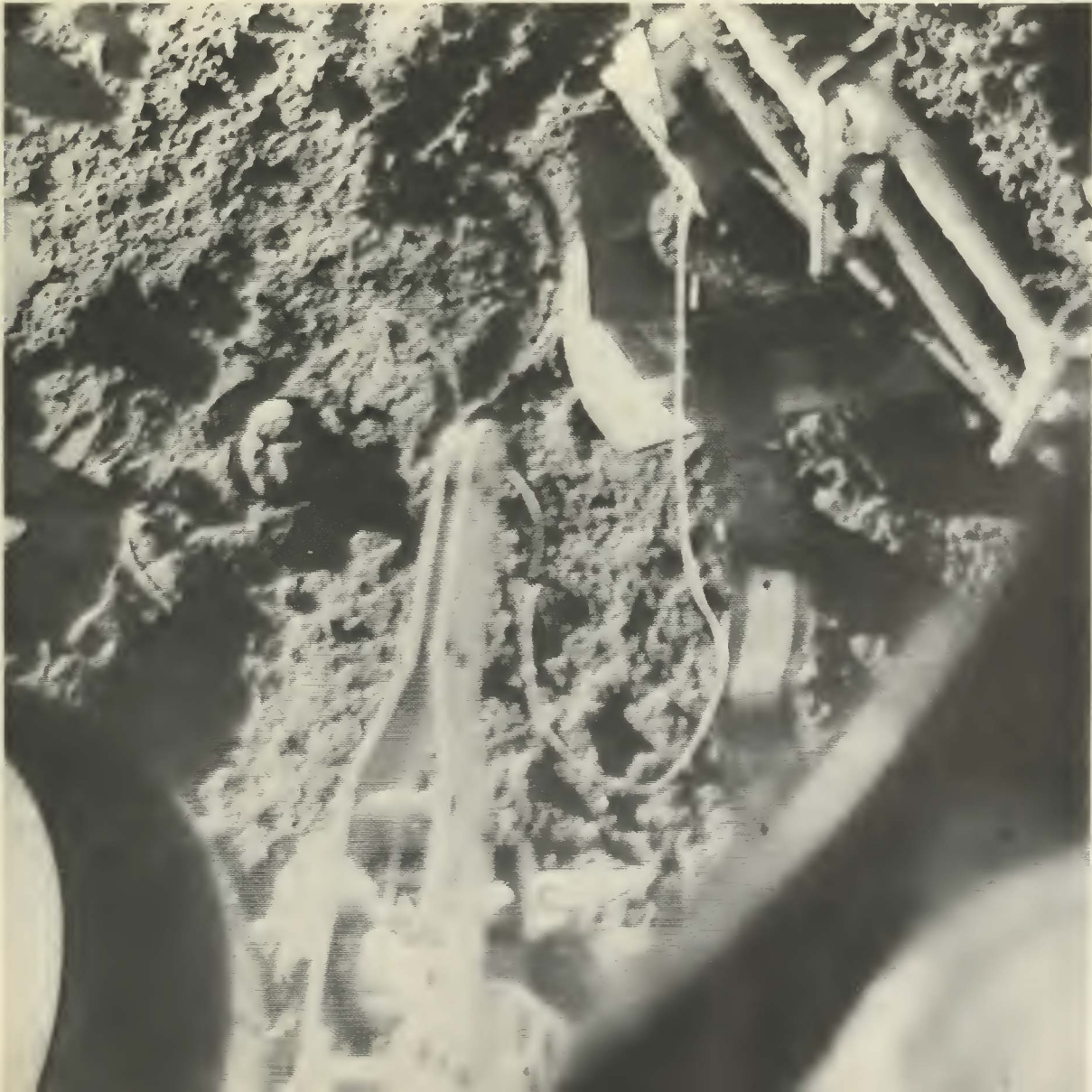
FIGURE 5-6.—Surface sampler holding the alpha-scattering instrument during deployment to third lunar sample on the Surveyor VII mission (day 022, 11:21:12 GMT).
