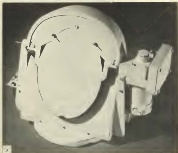
FIGURE 3-2.—Mirror assembly of the Surveyor television camera. (a) Surveyor I television camera hood and mirror assembly. A small visor was added to the top of the hood on the Surveyor III camera. (b) Mirror assembly and redesigned hood used on Surveyors V, VI, and VII.
