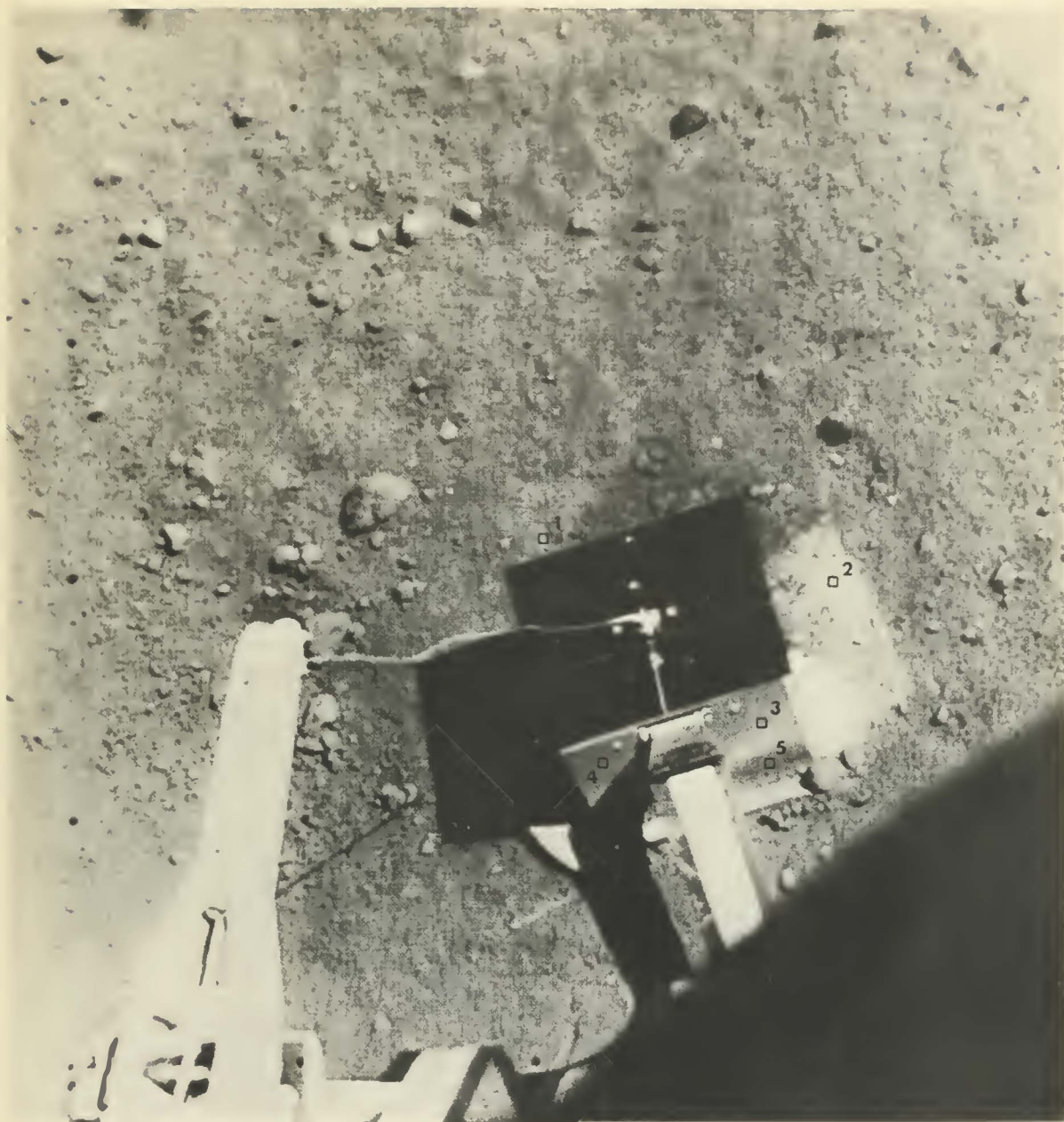
FIGURE A-2.—Wide-angle, digitized picture of Surveyor V sensor head and surrounding lunar surface, after engine firing. Squares and numbers indicate the areas selected for color determination. Taken through the green filter (Sept. 14, 1967, 03:55:43 GMT).
