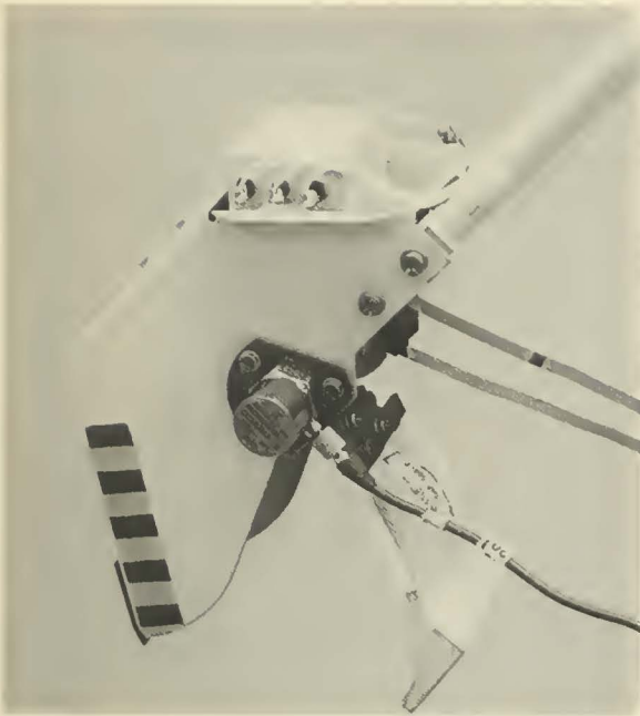
FIGURE 7-39.—Accelerometer attached to surface sampler to determine forces exerted on rock.
