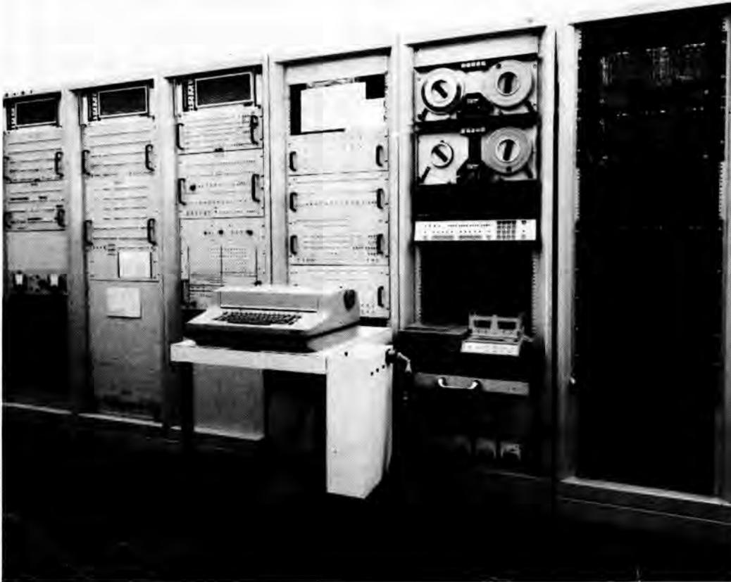
Figure 6-3. The Unified Data System: precursor to Galileo's Command and Data Subsystem. (JPL photo 360-630)
