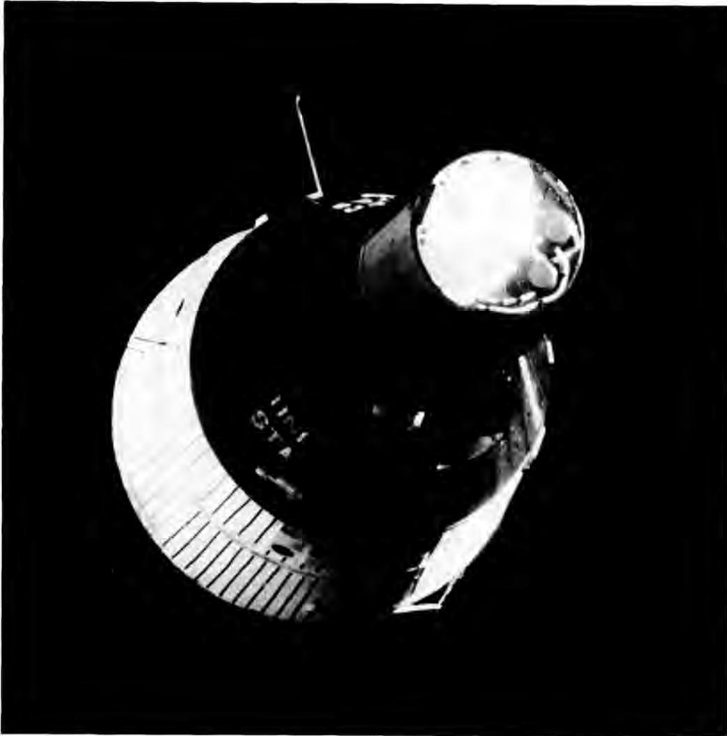
Figure 1-1. First orbital rendezvous: Gemini VI keeps station after using its on-board computer to maneuver to position near Gemini VII. (NASA photo S-65-63175)
