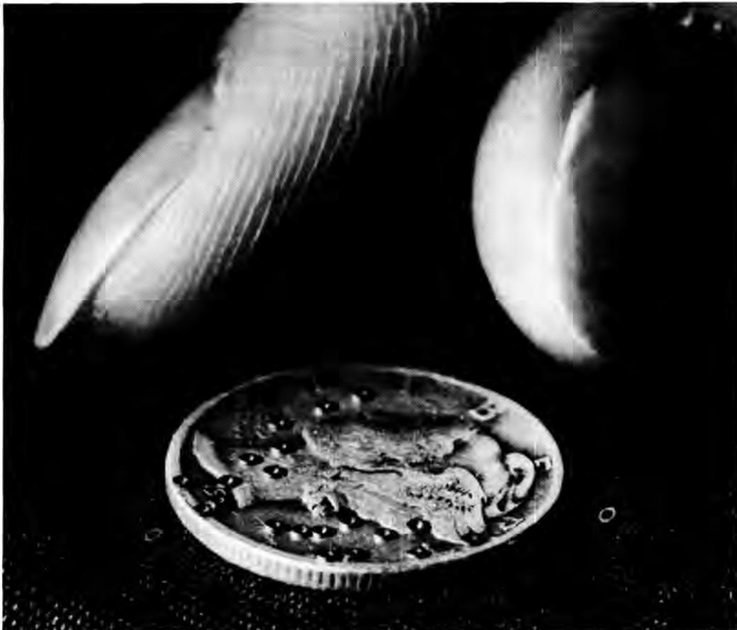
Figure 1-3. Cores like these were used in Gemini's memory. (IBM photo)
